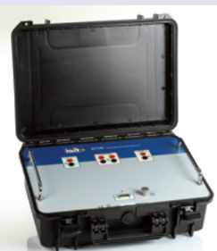
STDE POWER TRANSFORMER DEMAGNETIZER
